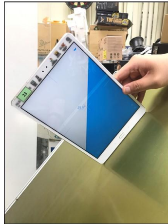
Figure 2. Angle measurement of inclined plane.
