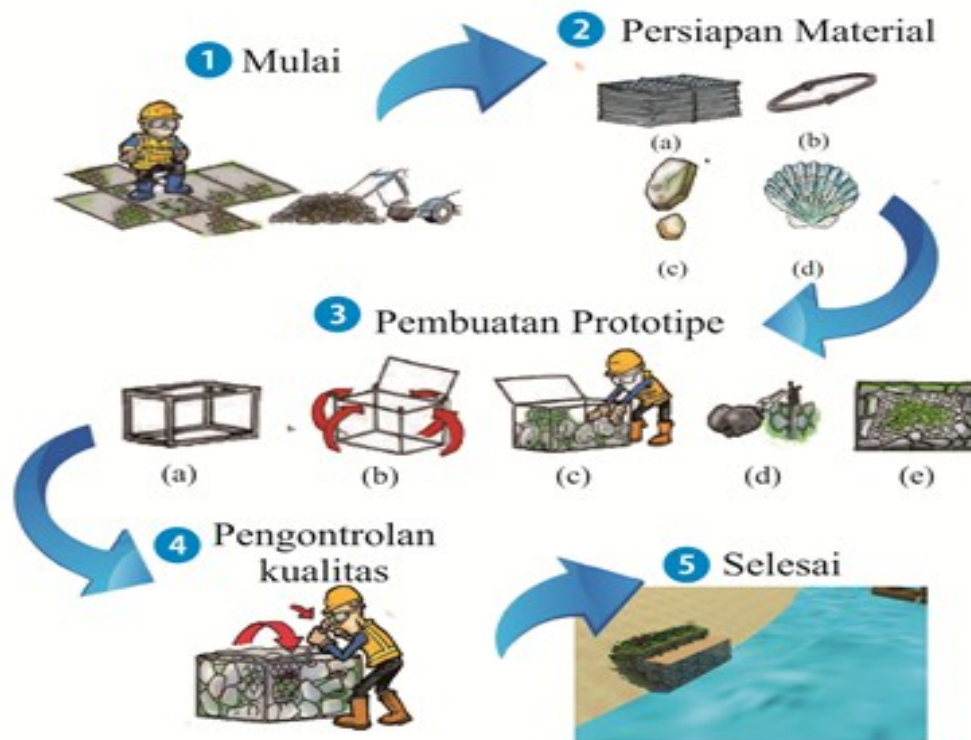
Gambar 3 Flowchart pembuatan prototipe gabion portable eco-friendly.
