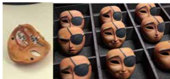
Figure 5. Over 23.000 3D printed faceplates were used in the production of Kubo and the Two Strings, each faceplate have their own specific codes.
