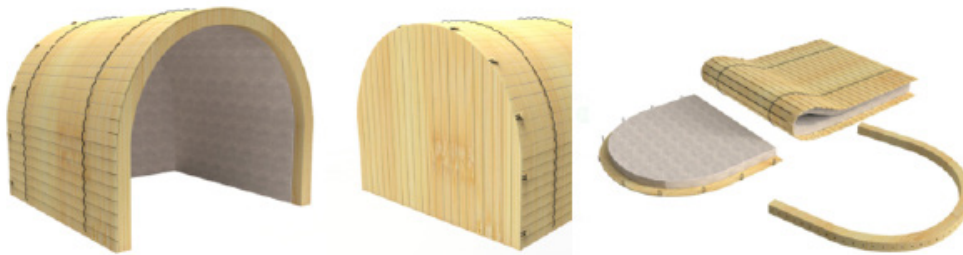
Image 6. Final Design Concept of Bamboo Soundproof Construction (Author, 2022)
