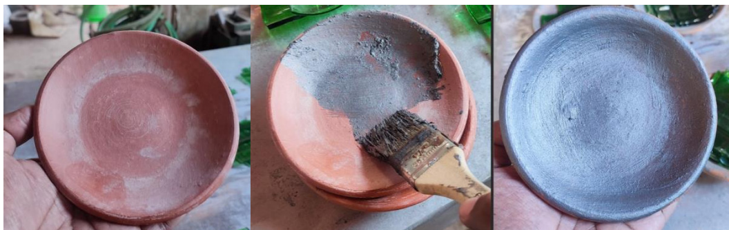
Image 3 Process of Coating the Mold with Separators. (Researcher, 2023)
