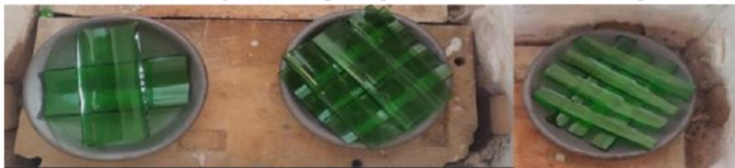
Image 4 Arranging the Mold in the Kiln. (Researcher, 2023)
