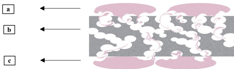
Figure 3. Process of bone in-growth into porous Ta scaffold. (a) The attachment of bone cells on the scaffold; (b) Pore size and porosity become a vital parameter to enhance bone in-growth; (c) The deep formation of bone
