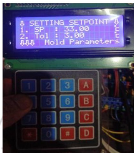
Figure 2 20x4 LCD Display with keypad for display commands
