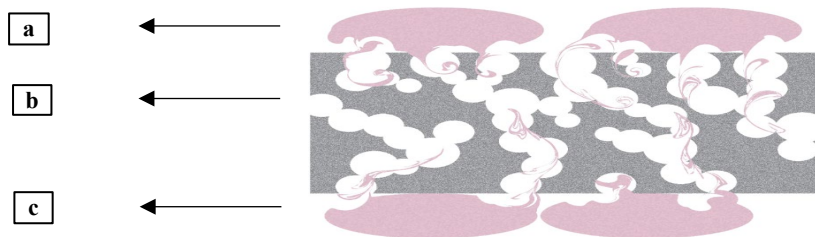
Figure 3. Process of bone in-growth into porous Ta scaffold. (a) The attachment of bone cells on the scaffold; (b) Pore size and porosity become a vital parameter to enhance bone in-growth; (c) The deep formation of bone
